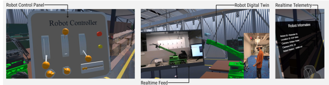
Figure 1: Operators can use RoboTwin via an extended reality application to control the robot wirelessly, with real-time updates and low-latency camera streaming.
